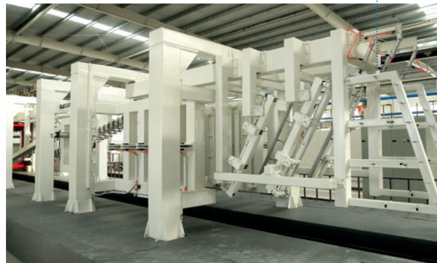
Grooving device with four sets of cutters that can be adjusted automatically without shutting down according to different grooving sizes (left) and surface cutting device (right).
