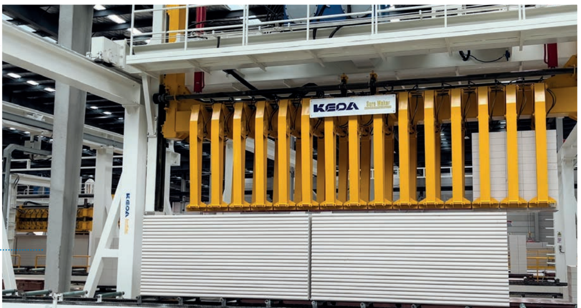
Clamping machine for panel and block transportation in the packing area.
