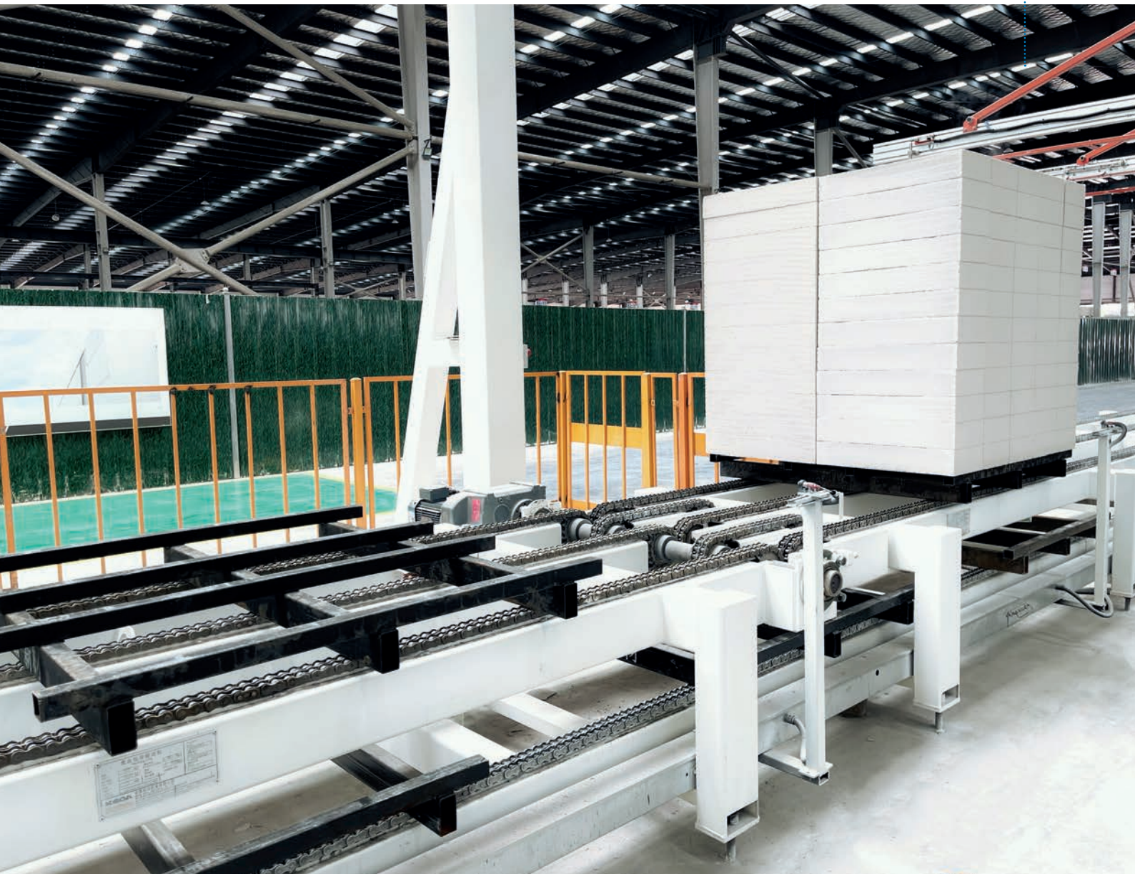
Double-layer conveyor for blocks and pallets.
