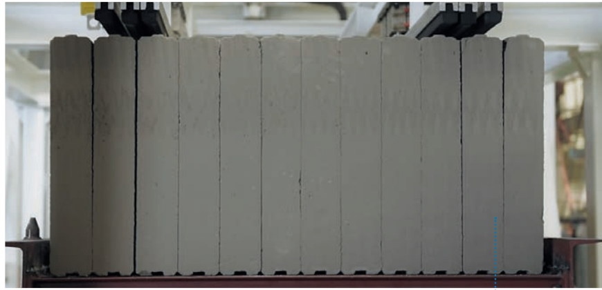
Green cake separation technology by Keda Suremaker.
