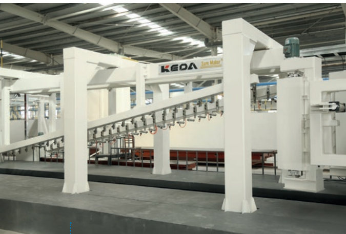
Cable-stayed horizontal cutting machine, each steel wire is fixed on a pair of independent wire hanging columns to avoid settlement cracks in the process of thin panel cutting.
